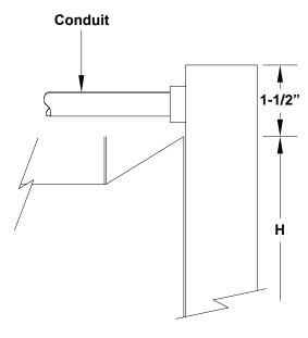
Stainless steel raceway mounted on exterior of hood. Raceway extends 1-1/2" above top of hood.
