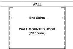
Top enclosures, back-splashes and end skirts mount with exposed sheet metal screws or rivets 18" on center, fasteners by others.
