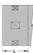
One Piece Construction When Building Entrance Is Large Enough And Neither "W" Exceeds 8 Feet Nor "L" Exceeds 12 Feet.
