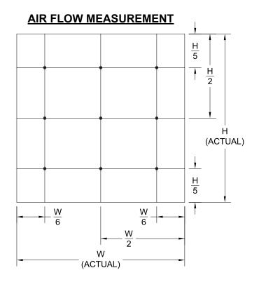
Velocity measured with Alnor Thermo Anemometer (Model 8525) with digital readout.
