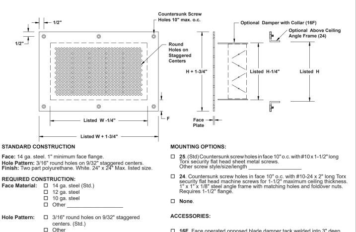
□ 16F. Face operated opposed blade damper tack welded into 3" deep collar that is stich welded to rear of face plate. Dampers are adjustable using flat bladed screwdriver.
