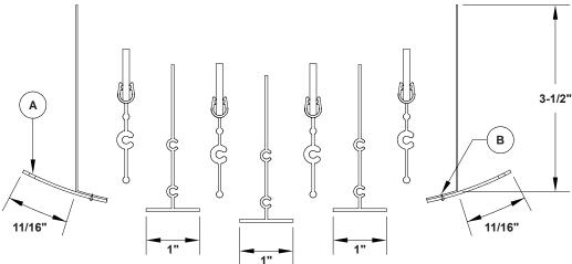
To fit all duct diameters from 12" to 60".
