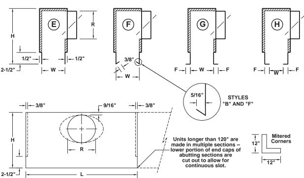
Material: 24 ga. galvannealed. Insulation: 1/2" standard. Other thicknesses available. Lengths: Any through 120" in one piece. Unlimited continuous length. Inlets: All sizes. Oval inlets available at an extra charge. Widths: 1/2" minimum - no limit on maximum. All sizes in between.
